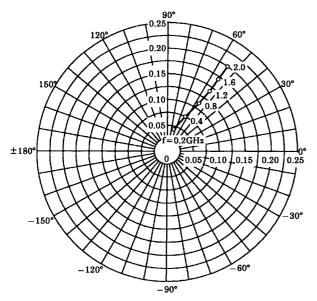
$S_{22e}$   $V_{CE} = 6V$   $I_{C} = 3mA$   $T_{a} = 25^{\circ}C$
